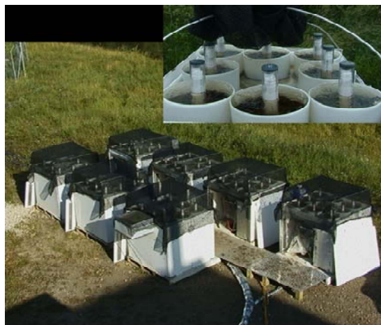
Figure 8-2: A) Small microcosm system with streams situated on tables over mixing reservoirs used in the Thompson River, British Columbia. B) Modular mesocosm system with streams situated on tables over mixing reservoirs used in the Little River, New Brunswick; Junction Creek, Ontario; the Wabigoon River, Ontario; and Key Lake, Saskatchewan
